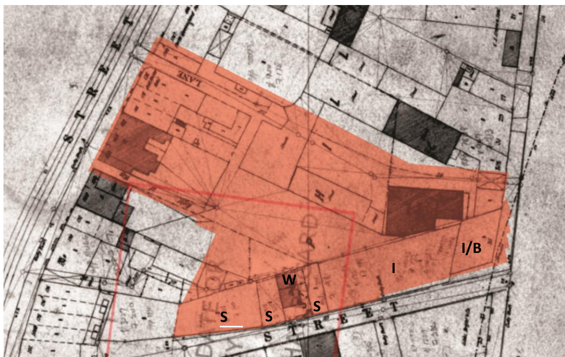
Figure Error! No text of specified style in document..1: Part of a Public Works Department survey dated from c.1893 with additions that date to 1900 showing construction materials of Underwood Street workshops and stores. Key: stone (S), timber (W), iron (I) and brick (B). Newer buildings are shaded black. PWDS1544-S1080, c.1893-1900, Sydney Water.
